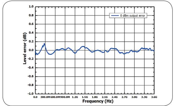
Measured at -20 dBm, level error vs. frequency
